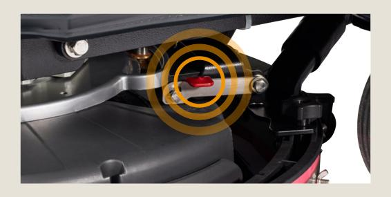
Lift the squeegee up by hand until it locks in the UP position, and turn off the vacuum, to perform double scrubbing.
