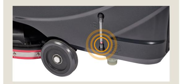
You can check the level of the solution anytime using the red ball on the left side of the machine.
