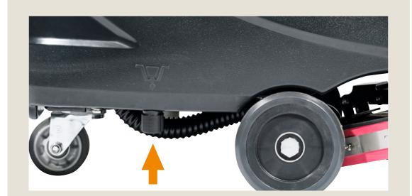
**Daily:** Empty the clean water tank using the solution tank drain knob under the machine.
