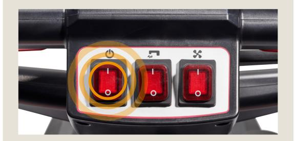
When scrubbing is complete, turn off the on/off button to perform the following maintenance.
