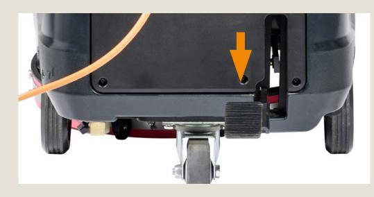
Lift the deck and squeegee by pressing the pedal down and to the left.
