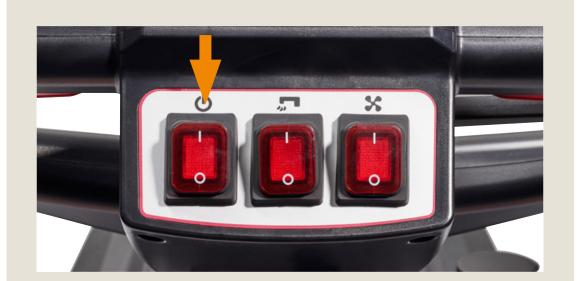
Connect the power cord to a 3-prong grounded electrical outlet. Press the machine ON button.
