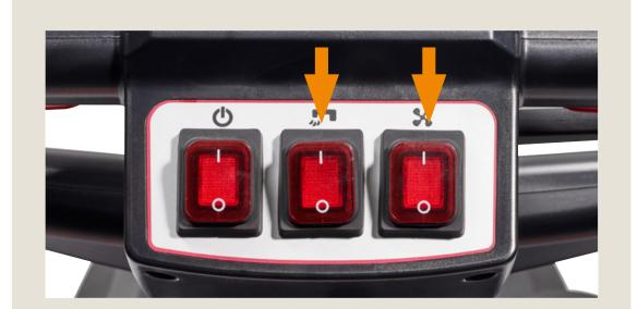
Press the solution and vacuum ON and start cleaning by placing your hands on either of the safety switches.
