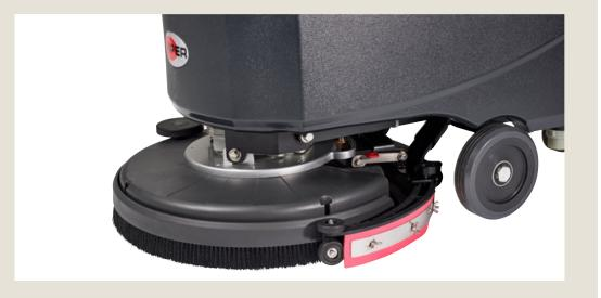
Install the brush or pad holder onto the drive plate and give a slight clockwise turn. Lower the brush deck by pressing the pedal down and to the right.
