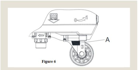
Solution flow can be adjusted to the scrubbing need by adjusting the manual valve located near the solution filter.
