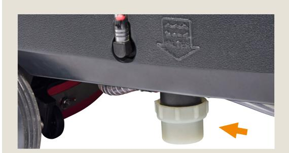
**Weekly:** Inspect the solution filter and clean if required.
